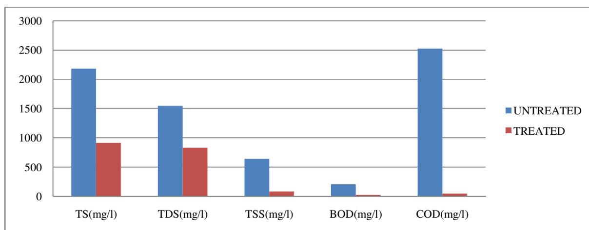
Fig 2- Graphical representation of percentage removal of the some studied physico- chemical parameters
