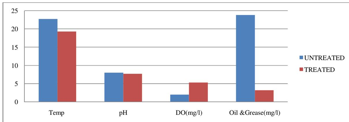
Fig 1- Graphical representation of percentage removal of the some studied physico- chemical parameters
